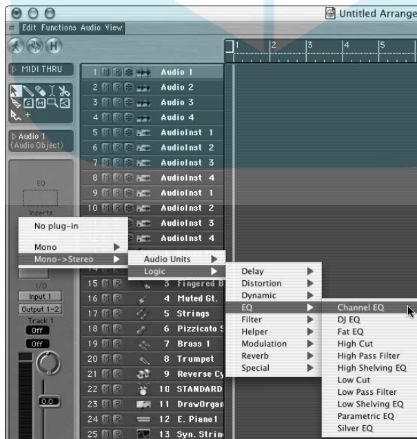
Figure 15-1: The Insert pop-up menu opens when you press the Insert input selector.
